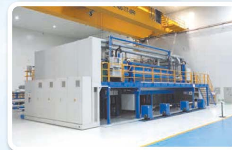
7.5 m Bushing Core Winding Machine
