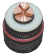
±535 kV copper conductor, XLPE insulated, copper wire shielded, laminated aluminum sealed, polyethylene sheathed DC power cable
