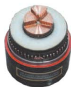
230/400 kV 1x2500mm 2 copper conductor, XLPE insulated, lead sheathed, polyethylene outer sheathed with temperature monitoring power cable
