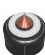
±535 kV 1x3000mm 2 copper conductor, XLPE insulated, corrugated aluminum sheathed, polyethylene outer sheathed DC power cable
