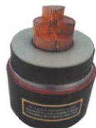
290/500 kV 1x2500mm 2 copper conductor, XLPE insulated, smooth aluminum sheathed, polyethylene outer sheathed Class C flame retardant power cable
