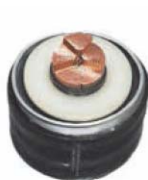
290/500 kV 1x2500mm 2 copper conductor, XLPE insulated, corrugated aluminum sheathed, polyethylene outer sheathed power cable
